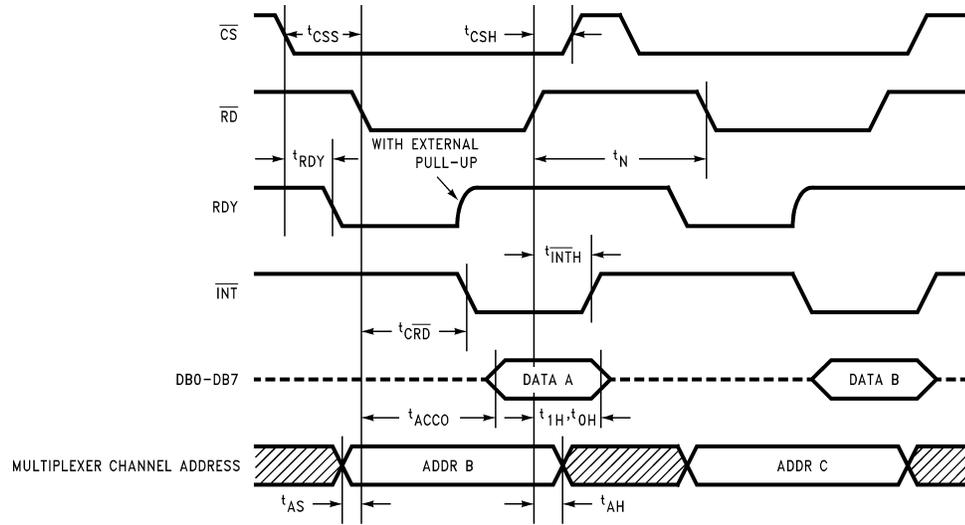
FIGURE 1.  $\overline{RD}$  Mode (Mode Pin is Low)
